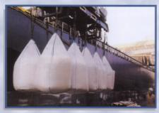
Interested in lowering your bag and packaging costs? Portabulk is the way to go. The Portabulk design uses all of its fabric to generate strength instead of just using the lift loops as in traditional bag design. The Portabulk bag can hold 3,000 pounds of product with a 5 to 1 safety factor, allowing it to lift more weight with lighter material and lower bag costs.
