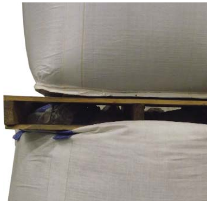
Standard Pallet Unprotected Entry, Potential bag Damage
